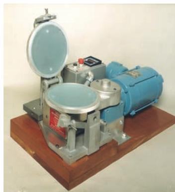
*The Hoover Automatic Muller provides a quick and easy method for preparing a small sample of pigment-resin dispersion. Glass plates that shear the pigment into the resin are easily cleaned by the solvent used in solubilizing the resin. This piece of equipment continues to find new uses wherever incoming pigment quality is a concern.*
